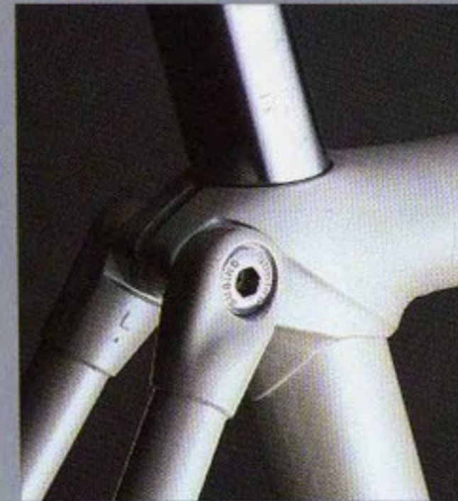
APA bonded investment-cast lugs work beautifully to resist the stresses of vibration.
