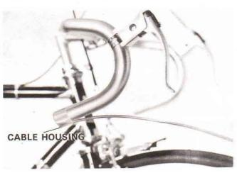
Step 2. Position one of the long cable housing on the bottom of the end of the handlebar with a peace of Scotch tape.
