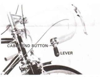
Step 6. Install cable through lever, mounting body and cable housing.
