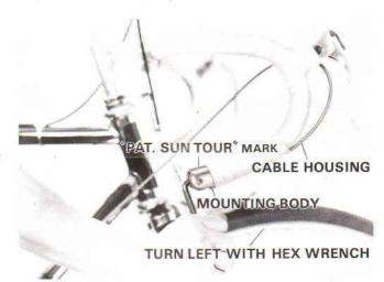
Step 4. Insert mounting body, keeping "PAT. SUNTOUR" mark facing upward, into end of handle-bar securing the excess tape.
