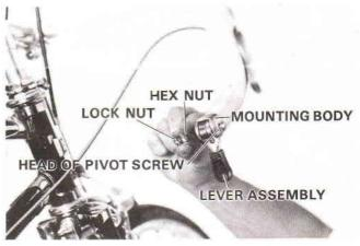
Step 5. Replace lever assembly into mounting body and fix pivot screw.
