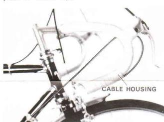
Step 3. Start handle bar tape on top of handlebar approximately 2" from handlebar stem. Tape around brake lever then begin taping cable housing to handlebar starting at approximately the first bend of the handlebar. Continue taping handlebar and housing and tuck any excess tape into end of handlebar.
